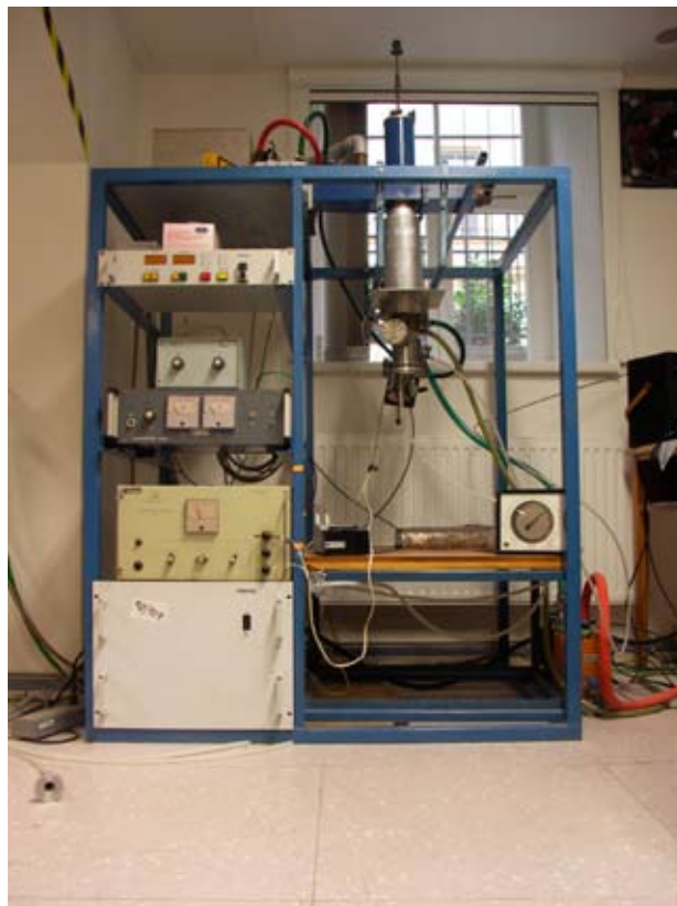
Fig. 2. Microwave ASTeX-type reactor used for UNCD deposition
