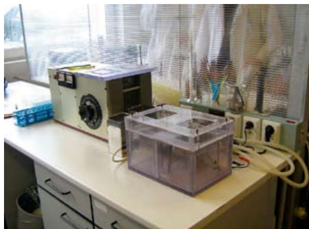
Fig. 1. Photograph of diaphragm discharge reactor used for decomposition of organic dyes dissolved in water
