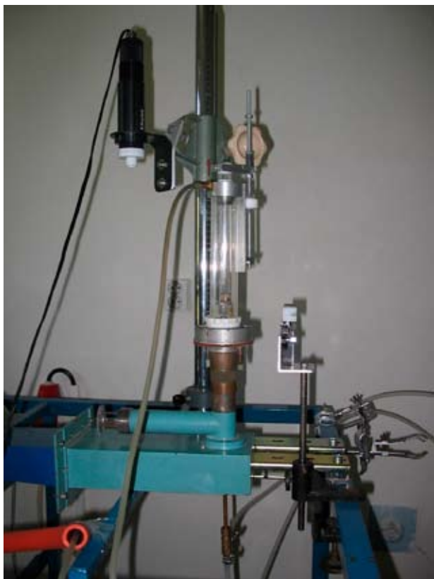
Fig. 1. Microwave torch used for synthesis of carbon nanotubes
