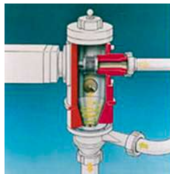
Fig. 2. Classifying cylindrical turbine of air classifiers
