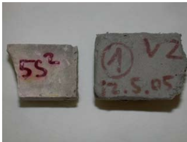
Fig. 3. Comparison of standard sample (left) without volume increase and sample T6vz with volume change
