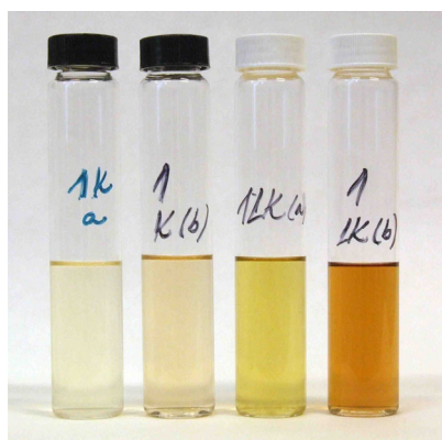
Fig. 3. Echinacea extracts (40 °C; K = roots; LK = leaves, blooms ; a = EtOH/water = 60/40; b = EtOH/water = 40/60)
