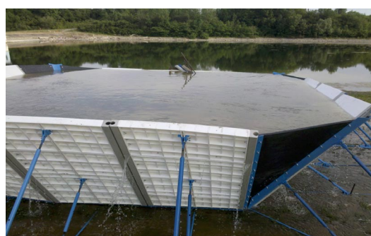
Fig. 7. “Pool” test for the verification of maximum hydrostatic load
