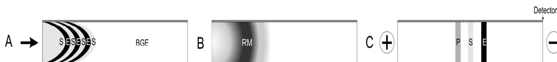
Fig. 1. Injection procedure. A – Injected zones. B – Creation of reaction mixture (RM) by diffusion. C – Separation of product (P) substrate (S) and enzyme (E)
